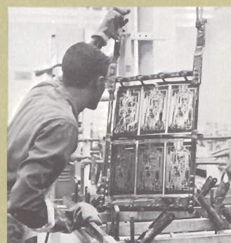
John Cannon checks on quality of printed circuit boards which have been copper plated in electrolytic baths.
