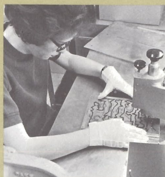
As one stage in the production of printed circuit boards, Charmane Arajakis drills holes to accommodate components.
